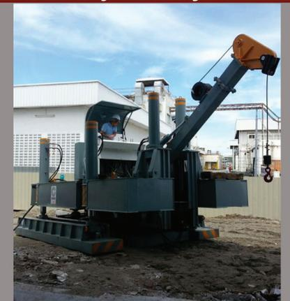
\*Able to pile inside factory / building with minimum heights of 2.8m and Maximum capacity up to 120 tons.
